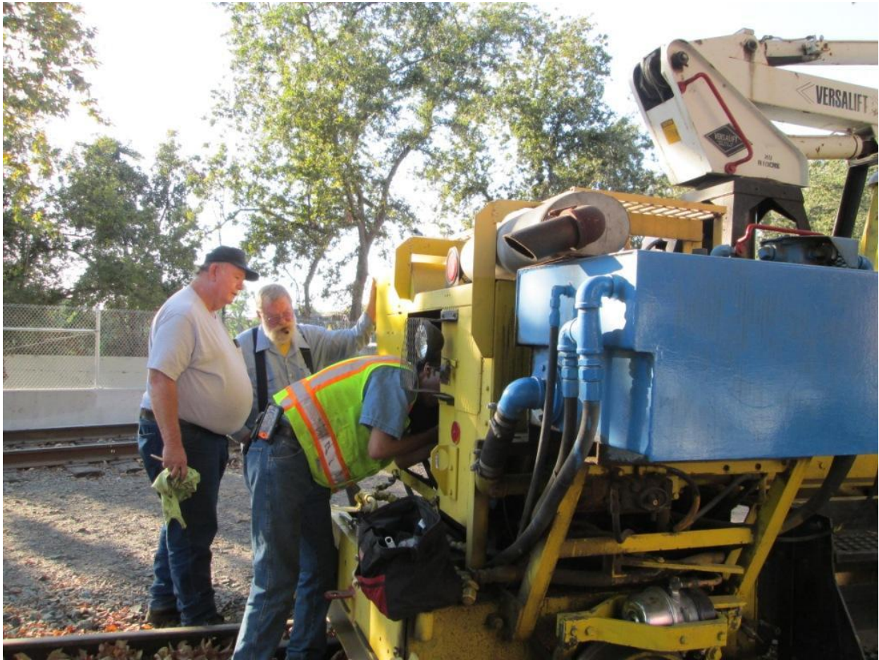
Gene and Pat providing supervision and guidance to Matt with the installation of the starter motor on the man-lift
